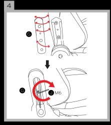
Mount the plastic covers onto the metal hinges using an M6 screw. The shape of the plastic cover should fit perfectly. Start with the left side.
