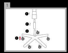
Install the wheels, gas lift piston and the piston cover onto the star base. These parts are easy to install. No screws, just click in place.
