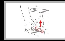
Lift the handle on the right side and lean gently forward or backward to adjust the position of the seat back/ top. Push down handle to lock the position.
