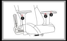
Lift the armrest: Press button (1) and pull the armrest upwards.
