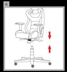
Insert the gas lift piston into the notch of the gas lift regulator underneath the seat. No screws needed, balance the seat and it will click in place. Gently apply pressure.
