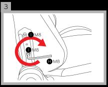
Use an M8 Allen key to fix the seat back/top onto the seat base metal hinges, using the same M8 screws.
