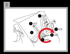
Mount the gas lift regulator underneath the seat using four M8 screws. It is important that the notch for the gas lift is mounted on the rear-end of the seat.
